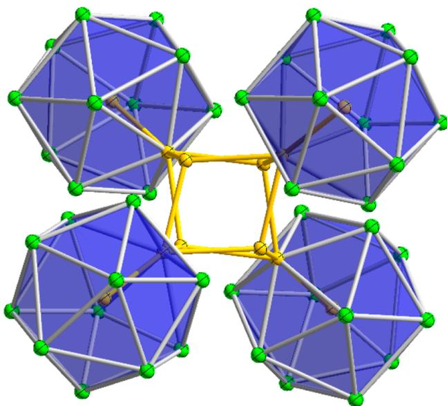
**Figure 11.** Crystal structure of the  $[\text{Au}_{12}\text{Pb}_{44}]^{8-}$  anion, where Pb is green and Au is gold.
