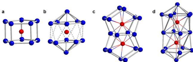
**Figure 4.** Crystal structures of  $[\text{Co}@\text{Ge}_{10}]^{3-}$  (a),  $[\text{Co}@\text{Ge}_{12}]^{3-}$  (b),  $\alpha$ - $[\text{Co}_2@\text{Ge}_{16}]^{4-}$  (c), and  $\beta$ - $[\text{Co}_2@\text{Ge}_{16}]^{4-}$  (d). Ge is blue, and Co is red.
