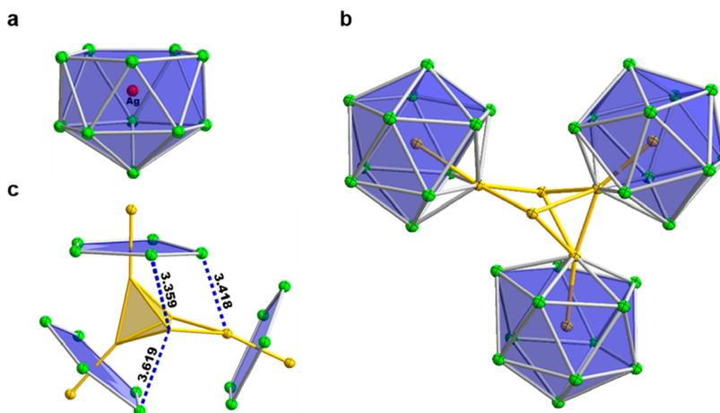
**Figure 10.** Crystal structures of  $[\text{Ag}@\text{Pb}_{11}]^{3-}$  (a),  $[\text{Au}_8\text{Pb}_{33}]^{6-}$  (b), and selected secondary  $\pi$ -type  $\text{Pb}\cdots\text{Au}$  interactions in the  $[\text{Au}_8\text{Pb}_{33}]^{6-}$  anion, with the secondary  $\text{Pb}\cdots\text{Au}$  contacts labeled (c).
