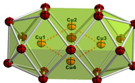
**Figure 7.** Crystal structure of  $[Cu_4@Sn_{18}]^{4-}$ , where Sn is dark red and Cu is brown.
