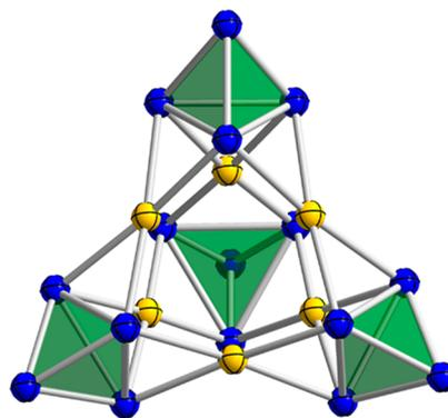
**Figure 1.** Crystal structure of the supertetrahedral clusters, [M<sub>6</sub>Ge<sub>16</sub>]<sup>4-</sup> (M = Zn, Cd), with Ge in blue and M in yellow.
